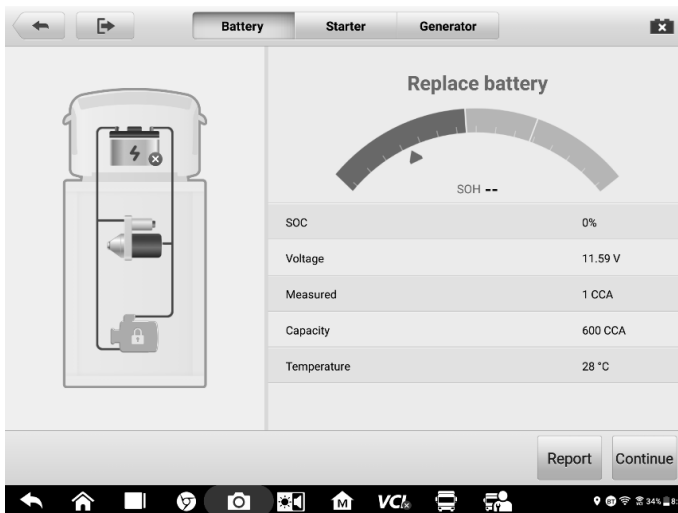
Figure 7-5 Sample Battery Test Results Screen
